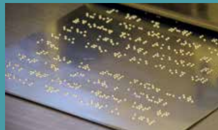
▲ In printing, a special braille paper is sandwiched and a roller is passed one by one on this Zinc plate
